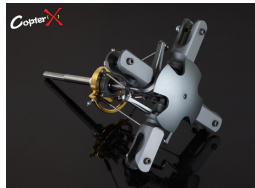
CopterX (CX600BA-01-20) 3D FLOATING Four Blades Main Rotor Set for 600 Heli
